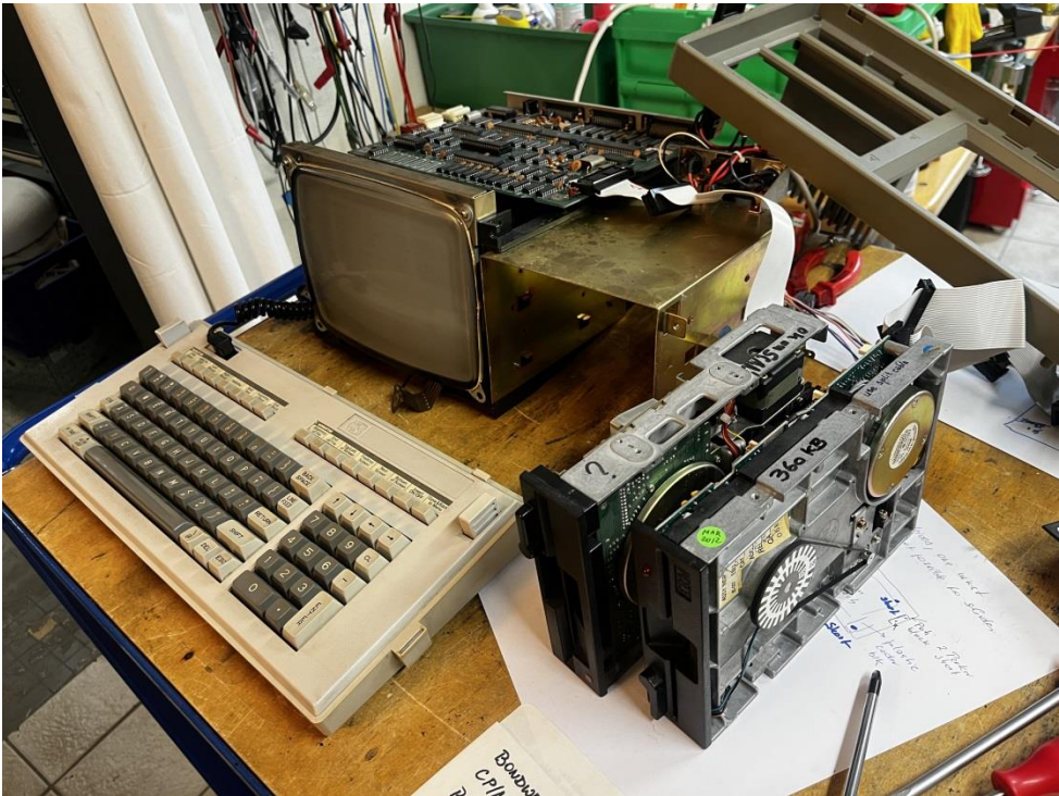
Fig.5. Tests with the replacement DSDD drives.
