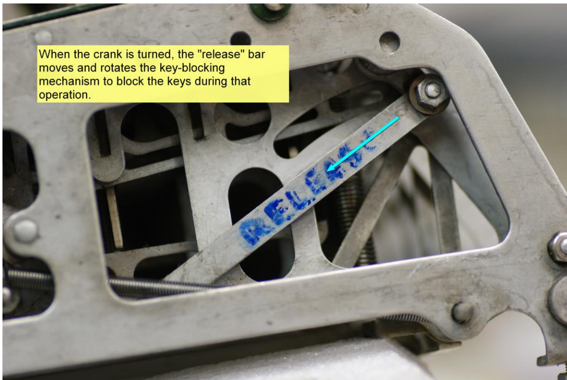
Fig.11: Lever pulled down in the direction of the blue arrow to rotate the key blocking axis
