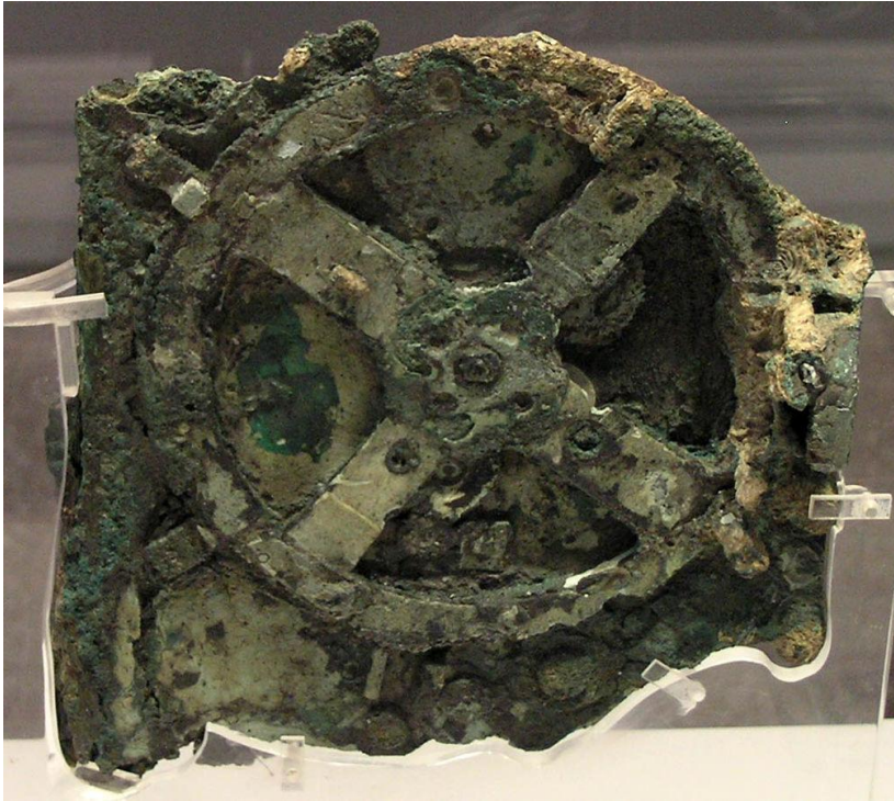
Antikythera, 78 BC (astrolabe) Oldest analog computer known: at least 30 gears! (found in 1900 by sponge divers)
