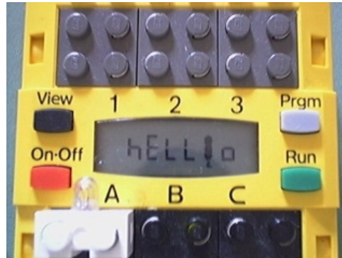
Figure 9: Improvised letters on a rudimentary LCD-display. “World” follows on a second screen.
