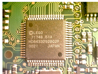
Figure 10: View on the H8/3292 microprocessor that controls the RCX.
