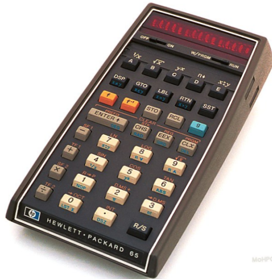
Figure 23: The HP-65 was the first programmable scientific calculator.
